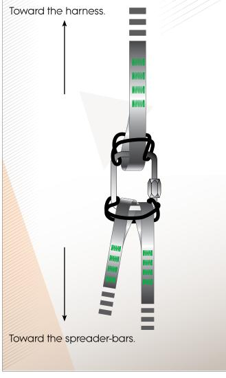
Connect the risers atop each spreaderbar (main hooking location), with the rectangular Inox ( stainless steel ) Maillons + the flexible elastic rings.
