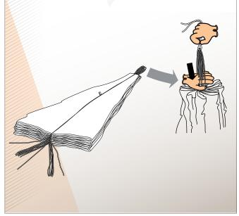
**4.a**. Push a line through the packing loops located at the center of the stitched lines on each panel at the balancing point between lines and central cord.
